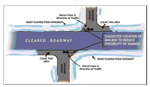
For un-curbed roadways, set the mailbox back at the far edge of the road shoulder to provide the maximum possible roadway clearance. For curbed roads, the face of the mailbox should be 8-12 inches back from the curb face.
